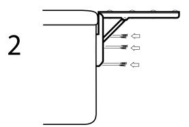
Secure each roller rack to the spa skirt by inserting all six #10 screws tightly into the screw holes that you marked in the previous step.
