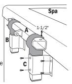
For spas with wide or irregular trim or 'picture frame' type cabinets, it may be necessary to insert a wood shim. When parts are in place and mounted to the spa cabinet, lock **B** and **C** together by drilling the 1/2" self-tapping screws into the holes provided on each Bracket C.
